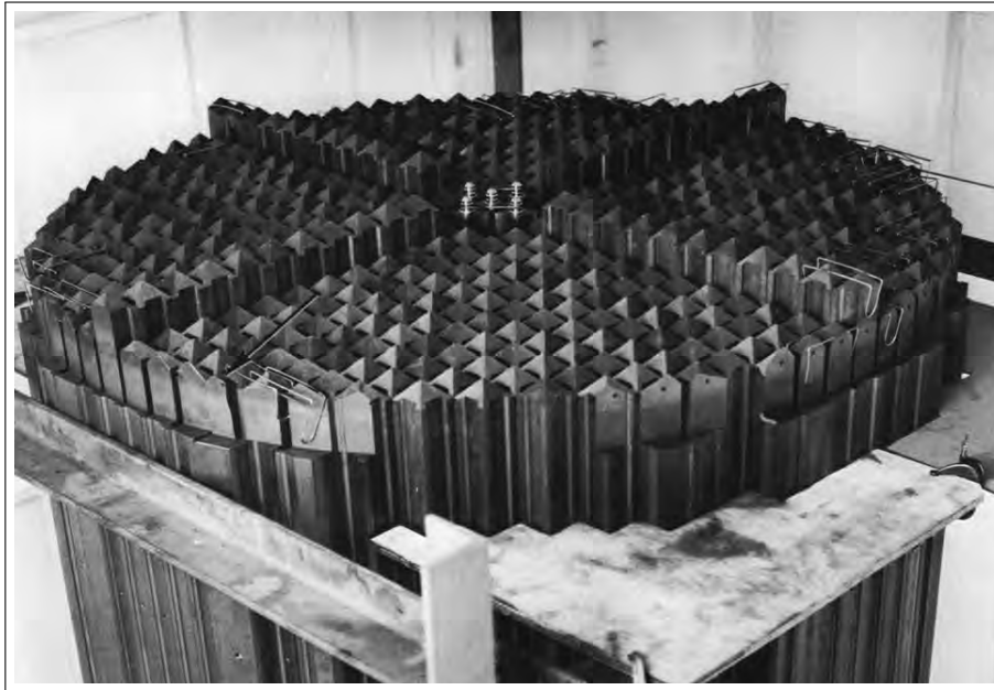
figure 27: top view of core assembly (rosenthal, briggs, and haubenreich 1971, figure 1.4).
